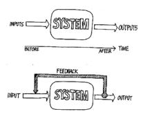
One example of feedback loop can be found in a thermostat. In order to keep a stable temperature in a room, it has a sensor that perceives changes; if the room is too cold, it sends a message to the furnace to produce heat, the effect of which is picked up by thermostat. A rise in the temperature will make the thermostat send another message to the furnace, making it stop. If temperature lowers anew, the cycle will begin again. This can be illustrated as follows:<sup>8</sup>
